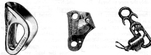
Left to right: Petzl Tibloc (12kN=2727 lbs) 8-11mm rope slips 4kN-7.5kN, Petzl Basic Ascender (12kN) 8-13mm rope slips 4.2kN-6.5k, Robot Friction Device (21kN) 6-13mm (rope fails before Robot slips)
